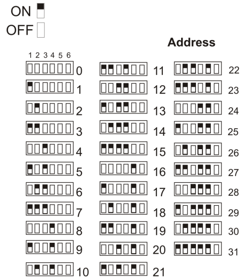
Figure 3: 5824 DIP Switch Settings Used to Set the ID Number
