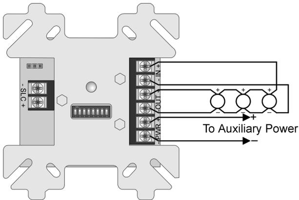
Figure 3: Class A (Style D) 2-Wire Detector Loop
