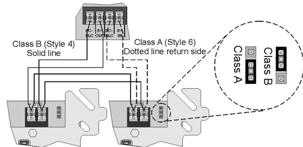
Figure 1: SLC Wiring
