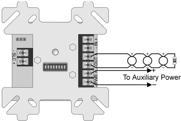
Figure 2: Class B (Style B) 2-Wire Detector Loop
