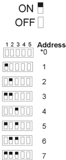
Figure 3. Set Dip Switches on the 5815XL
